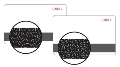
Card fingerprinting works by identifying the unique particulate pattern on a card's magnetic stripe as it is swiped through a Secure Card Reader Authenticator (SCRA).
