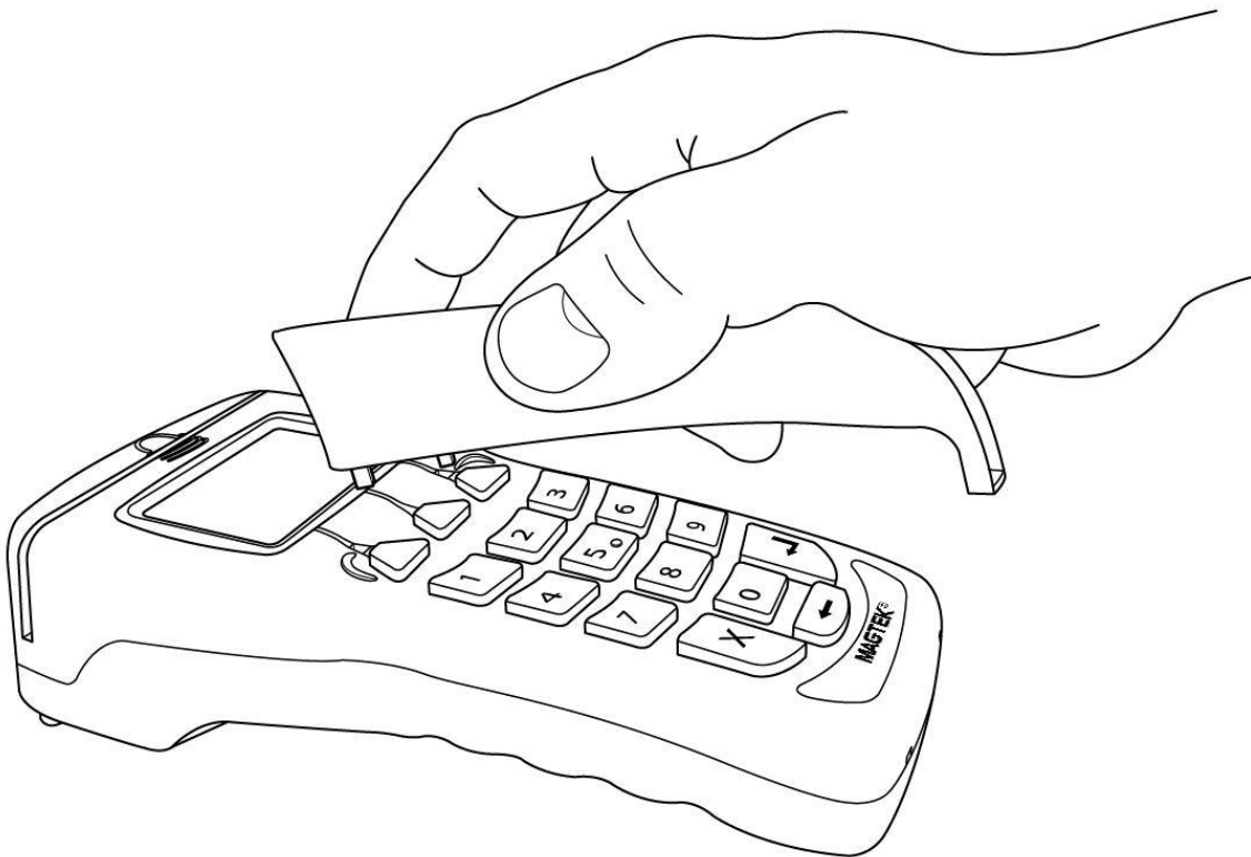
Figure 3-2. Installing the Privacy Shield
