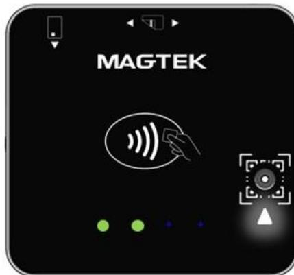
Figure 7-22 – BCR Transaction Bluetooth® LE Ready State
