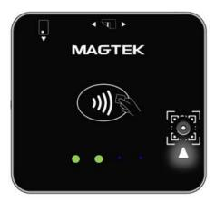
Figure 7-16 - BCR Transaction USB Ready State
