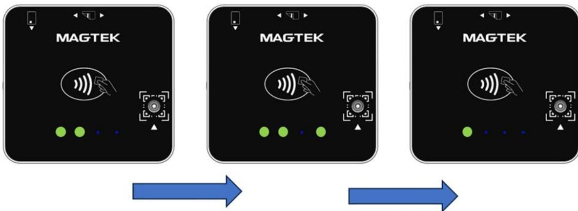
Figure 7-18 – LED Sequence – Payment Transaction Successful MSR Swipe (Connected via USB)
