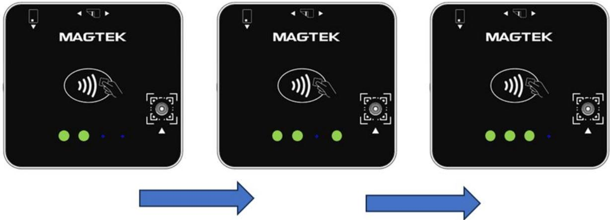
Figure 7-24 – LED Sequence – Payment Transaction Successful MSR Swipe (Connected via Bluetooth® LE)
