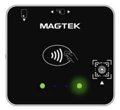
Figure 7-10 - Activate BLE Pairing Mode
