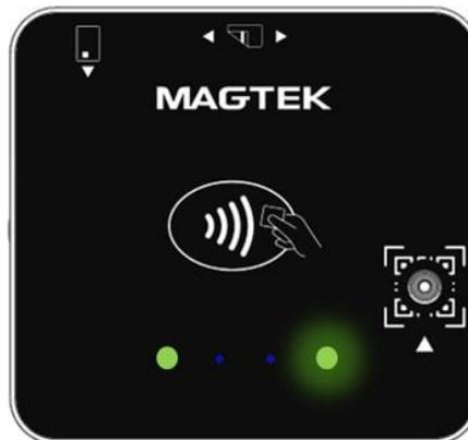
Figure 7-10 - Activate BLE Pairing Mode
