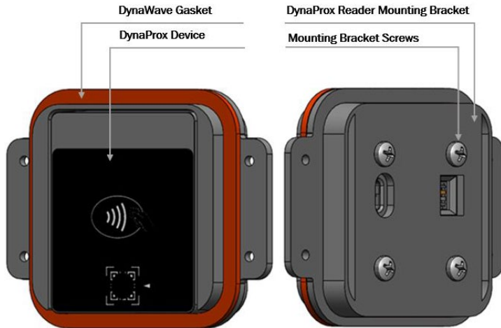
DynaWave to DynaProx (Shown Here) Conversion Kit Major Components - Fully Assembled
