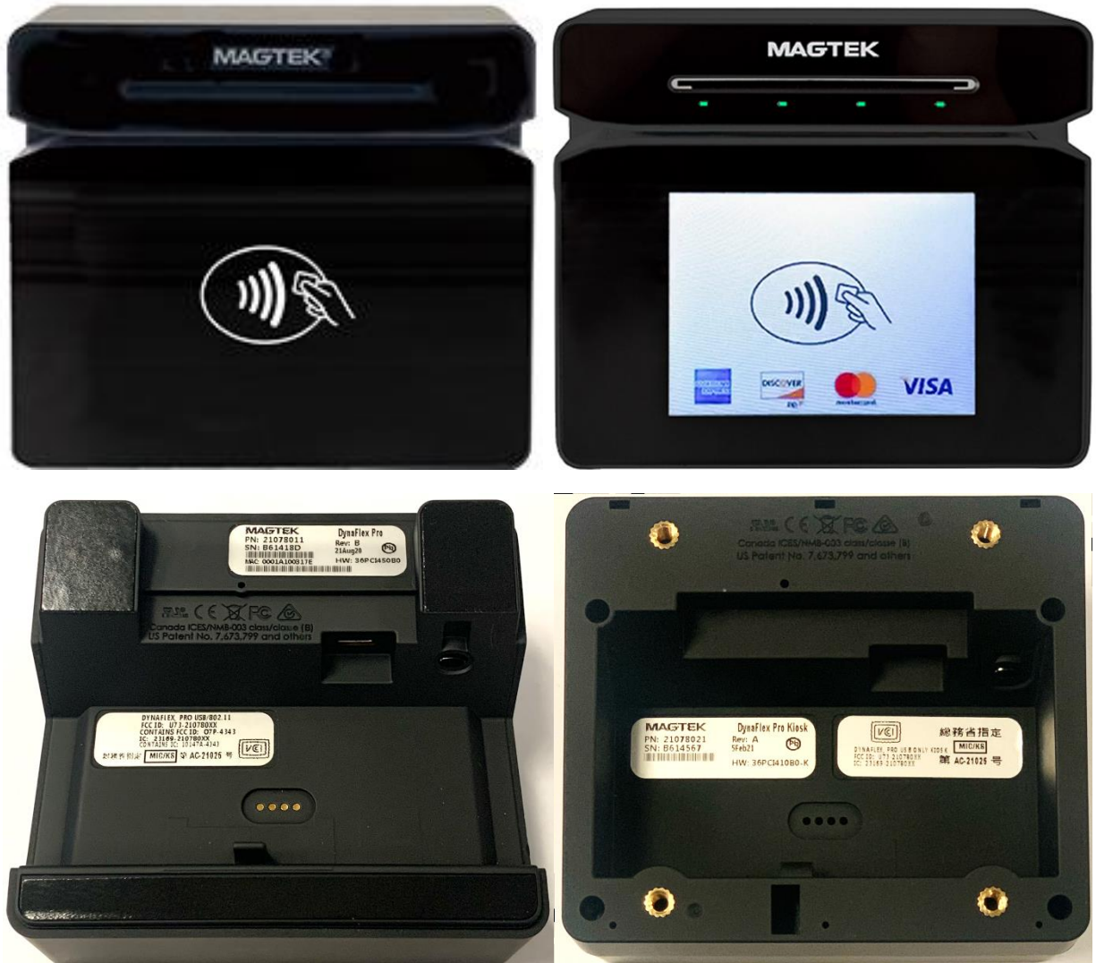
Figure 2-1 - DynaFlex Models Top View, DynaFlex Pro Models Top View, DynaFlex Models and DynaFlex Pro Models Bottom View, DynaFlex Kiosk Models Bottom View
