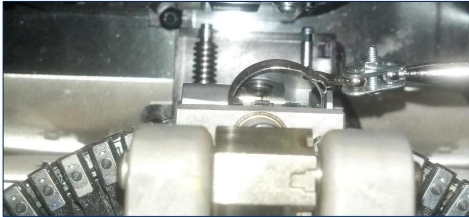
Figure 3-2 - Using Inspection Mirror to Check Tine / Hammer Alignment (TOP VIEW FROM FRONT)
