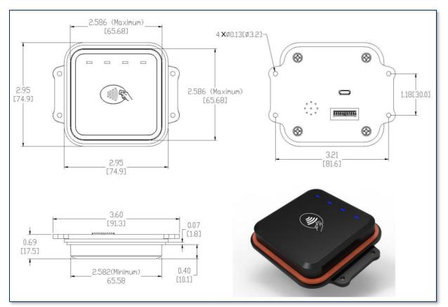
Figure 3-2 – DynaWave (Low Profile) Mechanical Dimensions in mm [inches]
