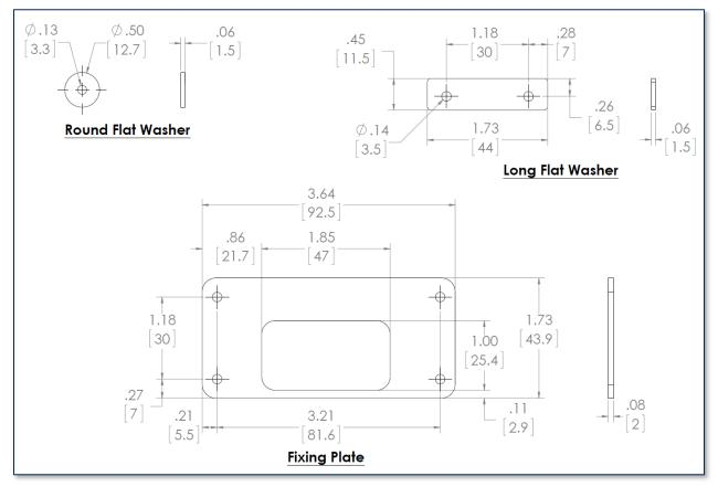
Figure 3-6 - Example Mounting Washer Designs
