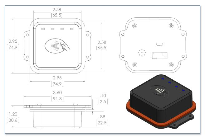
Figure 3-1 - DynaWave Mechanical Dimensions in mm [inches]
