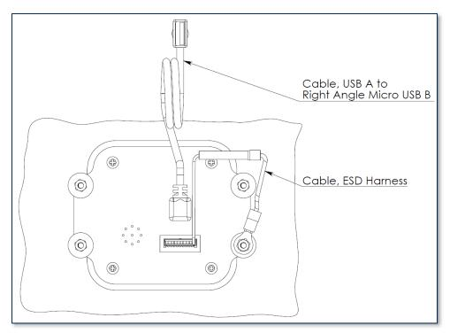
**Figure 2-1 - Cable Configurations for Earth Ground**
