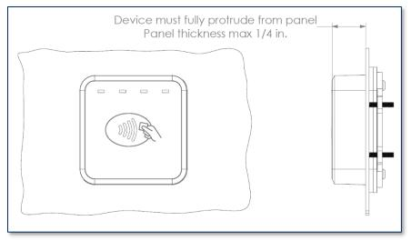
Figure 3-5 - DynaWave Protrusion from Panel
