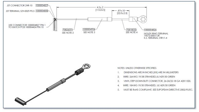
Figure 2-4 - Example Ground Cable
