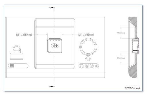
Figure 3-6 - DynaWave Protrusion Clearance Example
