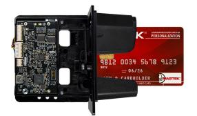
DynaDip Extended Bezel Secure card reader authenticator with magstripe and EMV contact card reading.
