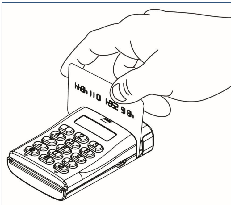
Figure 4-4 - Swiping a Card Through DynaPro Mini
