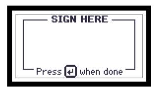
An error (0x8A) will be reported in ACKSTS of **Report 0x01** – **Response ACK** if the system is not available or the Touch Screen is not connected or doesn't exist.
