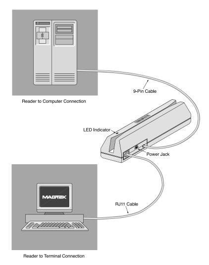
Figure 2-1. Reader Connections
