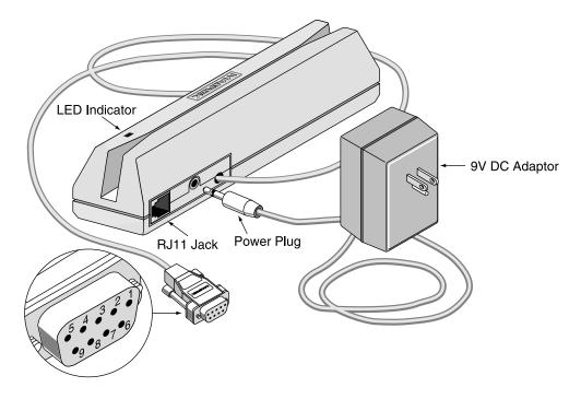
Figure 1-2. Reader Cable and Power Adaptor
