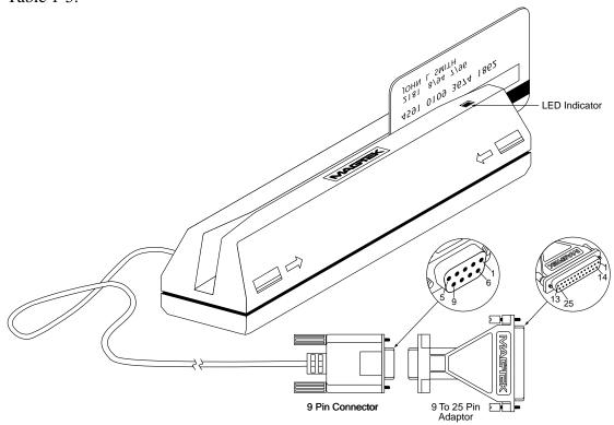
Figure 1-4 shows the Reader, cable and optional adaptor. Pin numbers and signals are listed in Table 1-5.
