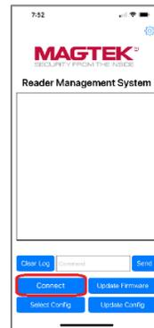
5. Tap on the **[Update Firmware]** button. Do not turn off your device or switch screens during the update process. Press **[OK]** Button.
