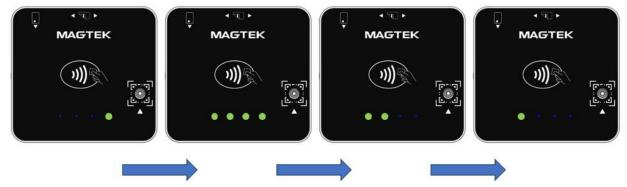
Figure 7-7 - Power On in Battery Operating Mode
