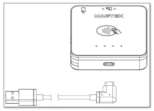
Figure 4-1 - Connecting to a Host via USB-C
