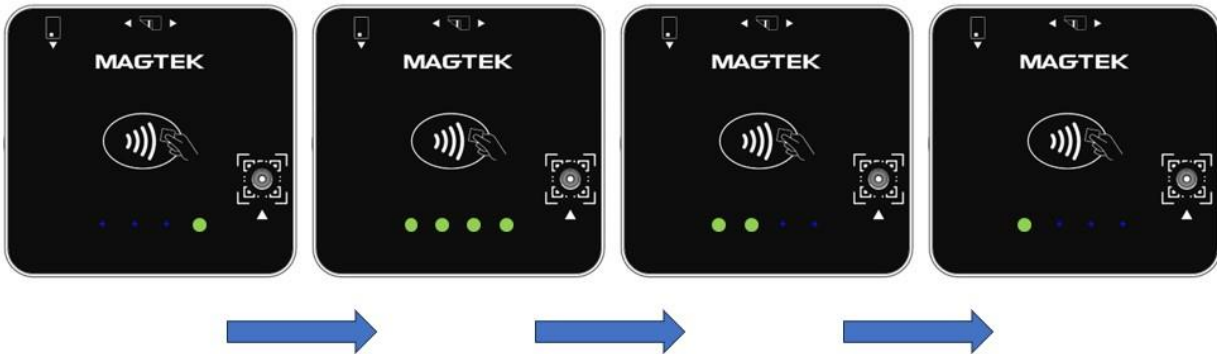
Figure 7-7 - Power On in Battery Operating Mode
