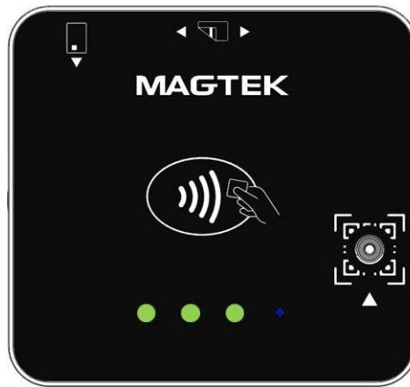
Figure 7-8 - LED Behavior for Bluetooth® Low Energy (LE) Ready State
