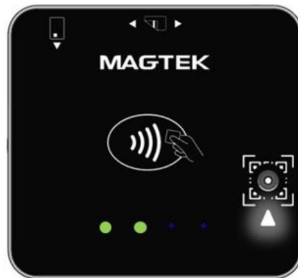
Figure 7-15 - BCR Transaction USB Ready State
