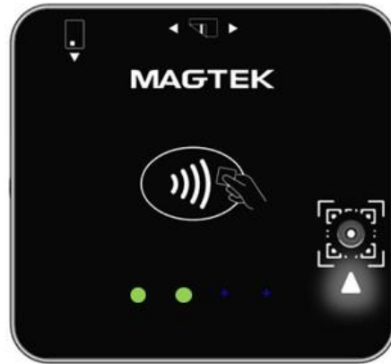
Figure 7-21 – BCR Transaction Bluetooth® LE Ready State
