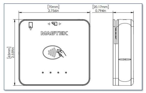
Figure 4-5 - DynaFlex II Go Overall Dimensions
