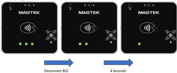
Figure 7-14 - Bluetooth® LE Disconnect LED Sequence
