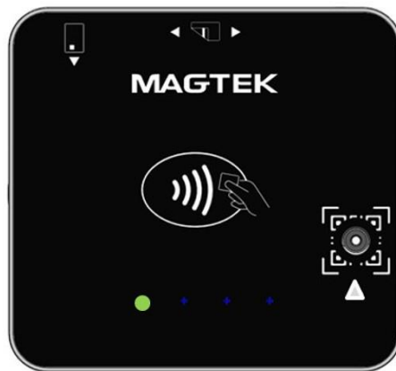
Figure 7-22 – BCR Transaction Barcode Detected (Connected via Bluetooth® LE)
