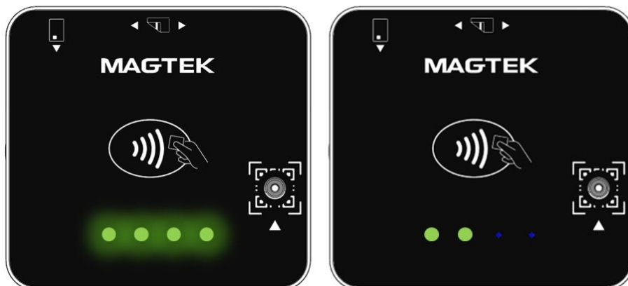
Figure 7-5 - LED Power on Sequence - USB Power On
