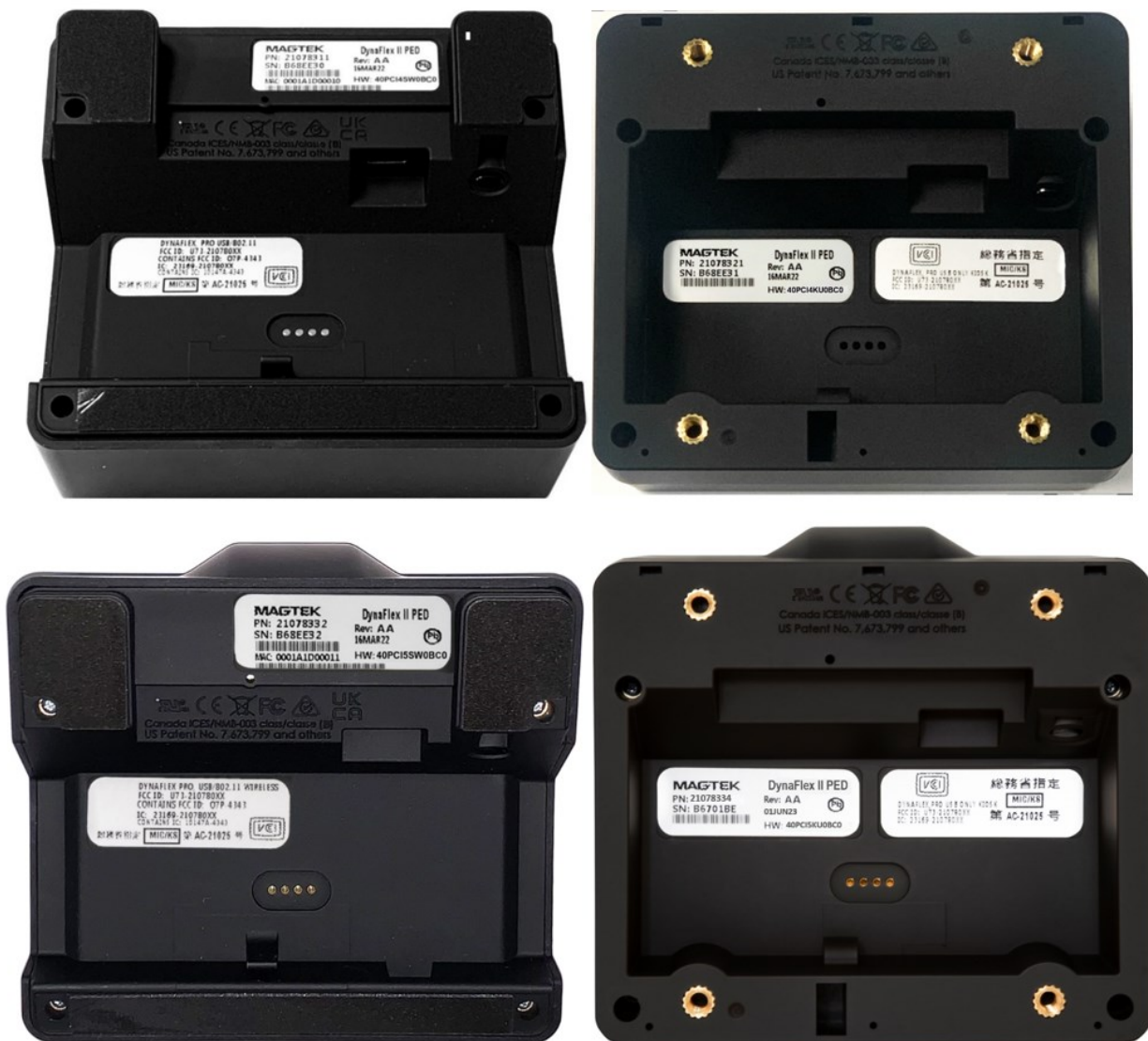
Figure 2-2 - Bottom views of DynaFlex II PED, DynaFlex II PED (Kiosk), DynaFlex II PED (BCR), and DynaFlex II PED (BCR & Kiosk)
