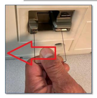
4) Continue pushing the tool to the left so it stays engaged with the right wall of the slot, and slowly pull the tool out, scraping the right wall of the card insertion slot clean as you pull.
