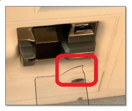
2) Push the tool straight into the card insertion slot all the way until you feel it touch the back wall.
