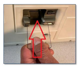
3) Push the butt end of the tool to the left. This pivots the tool inside the device and pushes the hook against the **back right corner** of the card insertion slot.
