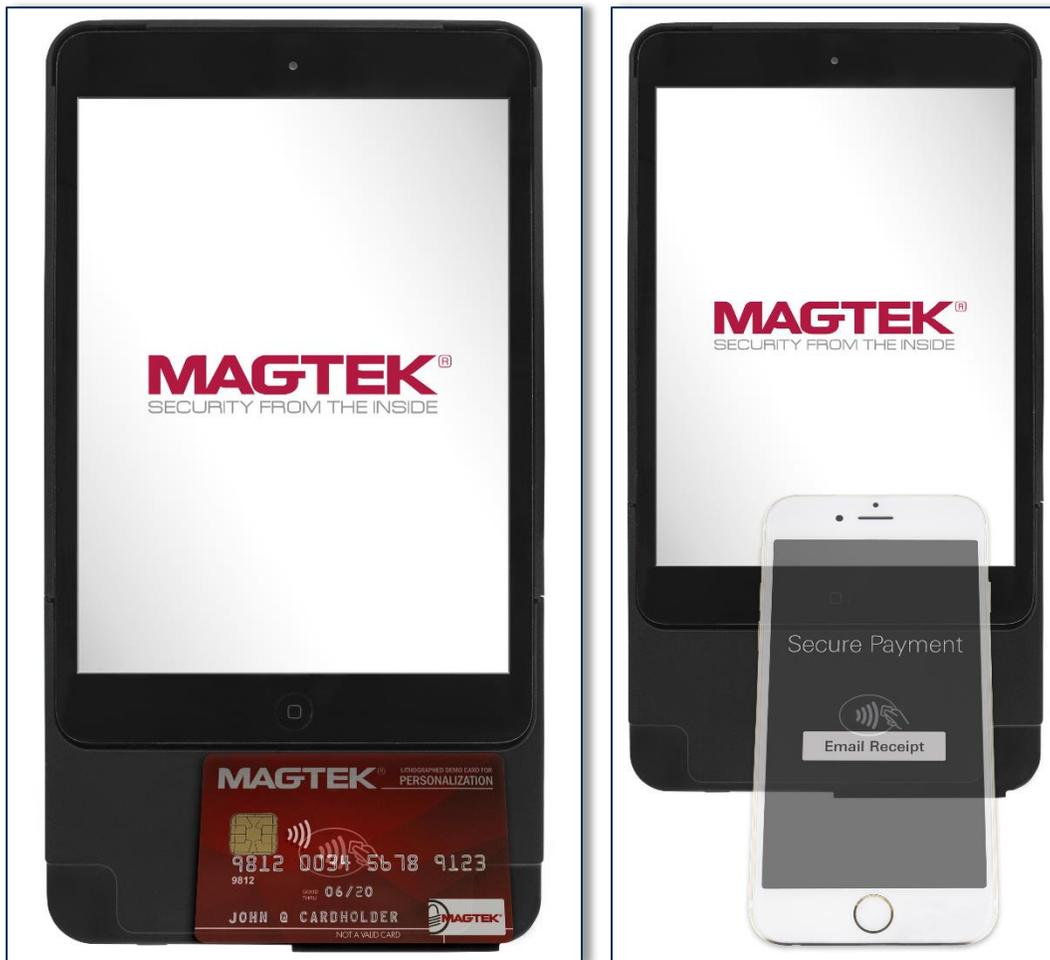
**Figure 3-3 - Tapping a Contactless Card or Smart Phone On kDynamo**
