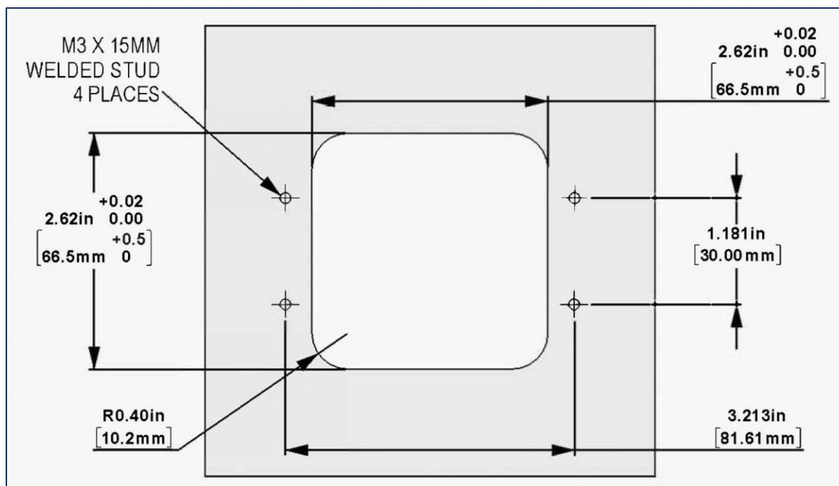
Figure 3-4 - DynaWave Panel Cutout Dimensions in Inches [mm]
