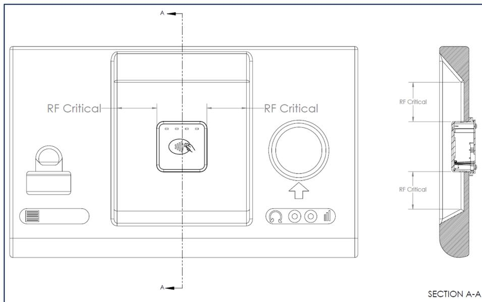
**Figure 3-6 - DynaWave Protrusion Clearance Example**
