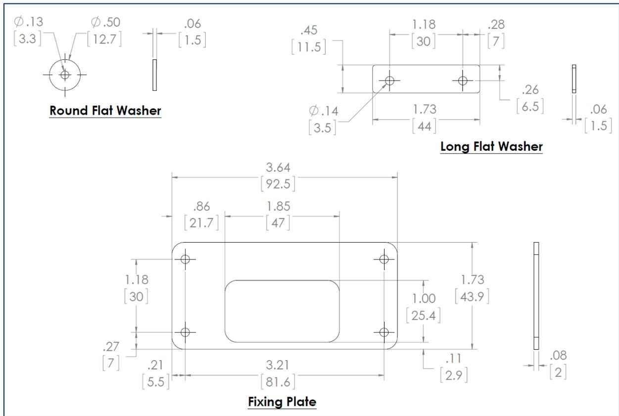
**Figure 3-6 - Example Mounting Washer Designs**
