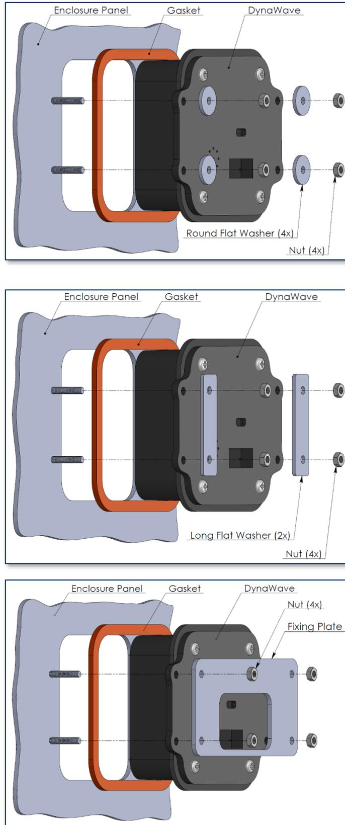
Figure 3-7 - DynaWave Threaded Stud / Nut Mounting
