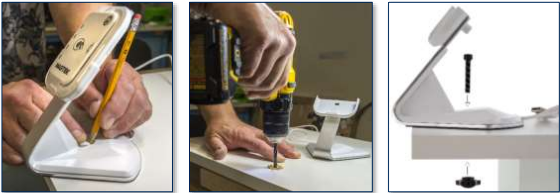
Figure 2-3 - Optional Docking Stand Assembly
