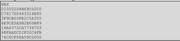
The host software can ignore the last two bytes because by definition MagnePrint data is 54 bytes long:
