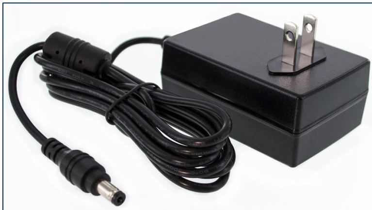
Figure 2-1 - Example Earth Ground Isolated 24V Regulated Power Supply
