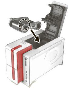
Install the ribbon. Ribbon drops into place (clips to the front of the device.)
