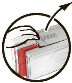
To Load ribbon: open the top access door (unlock if applicable).
