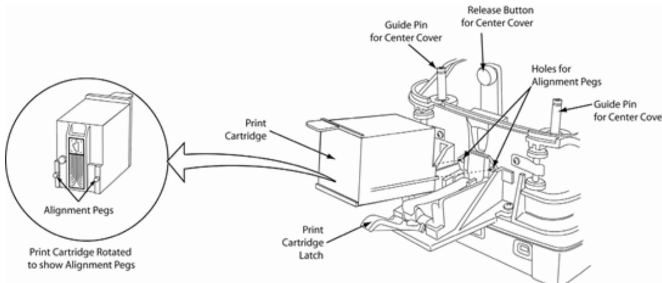
Figure 4. Rear Print Cartridge Installation/Removal
