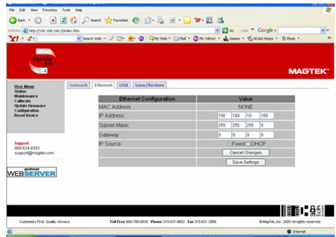
Figure 2. Ethernet Configuration Screen
