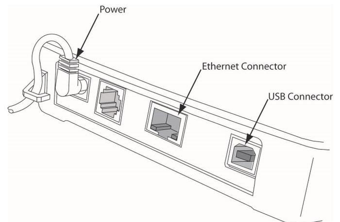
Figure 3. Cables & Connectors
