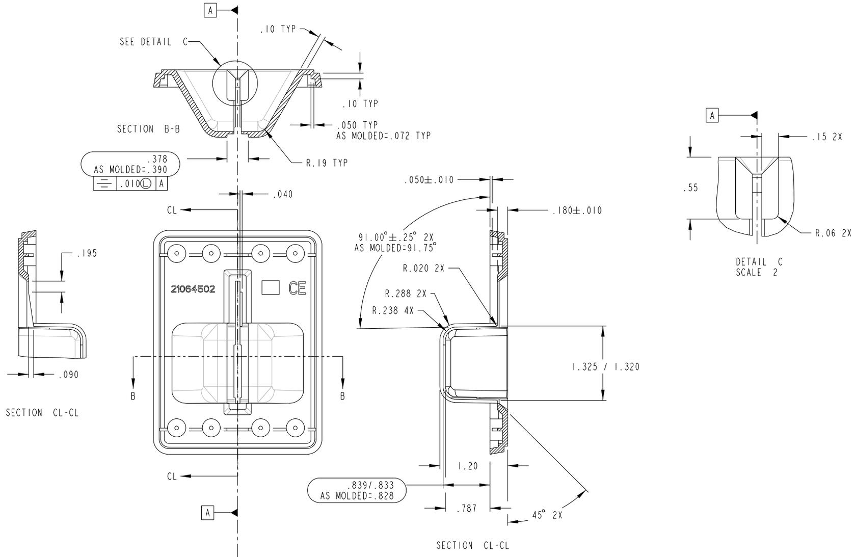
Figure B-2. Dimensions for Flat-Faced Bezel Design, Sheet 2
