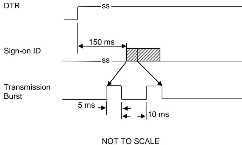
**Figure 3-1. Timing For ID Sign-on and Transmission Bursts.**
