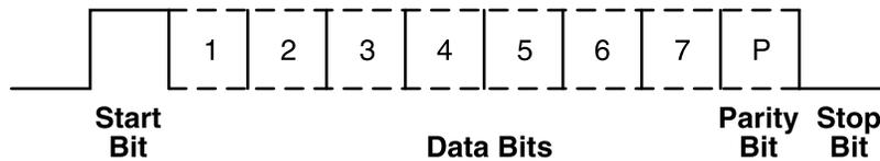
Figure 3-3. Transmission Timing
