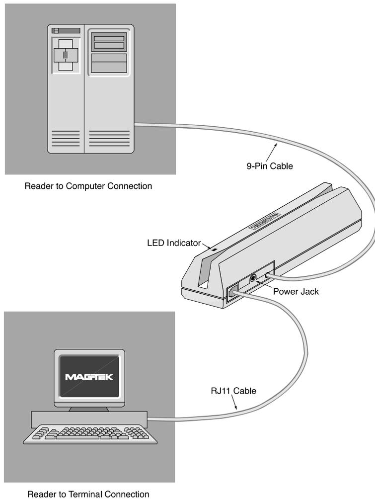
**Figure 2-1. Reader Connections**
