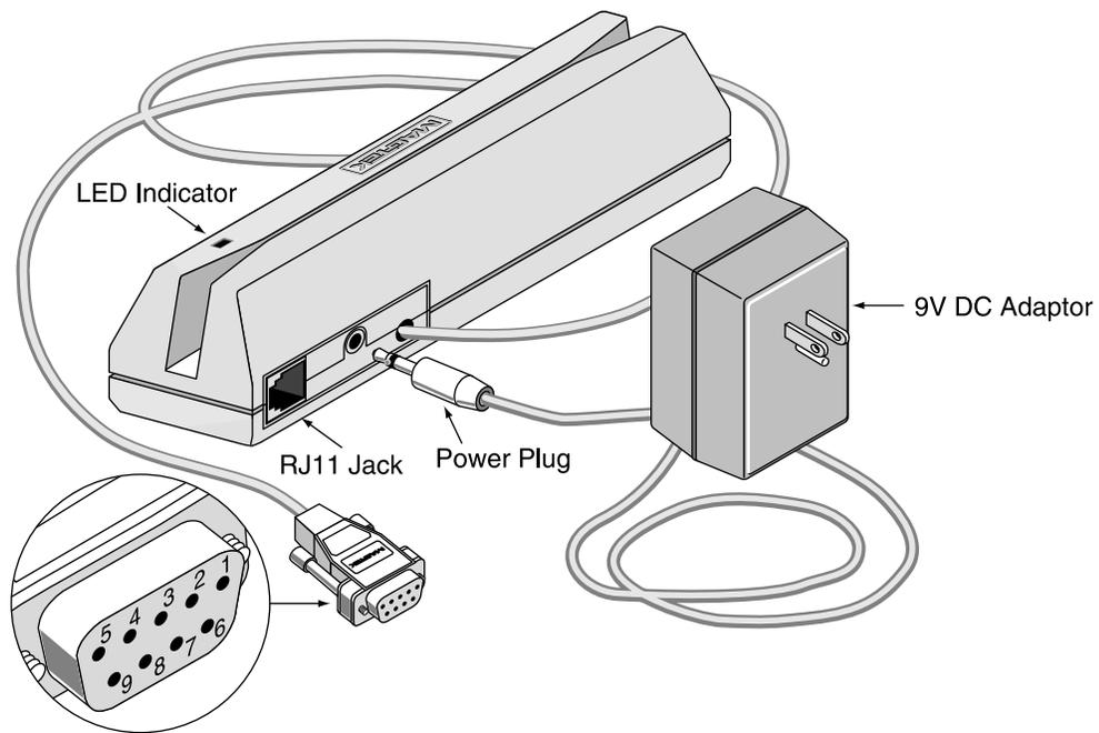
Figure 1-2. Reader Cable and Power Adaptor
