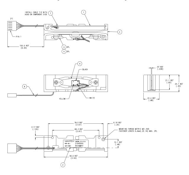
Figure 2-1. Reader Mounting Dimensions
