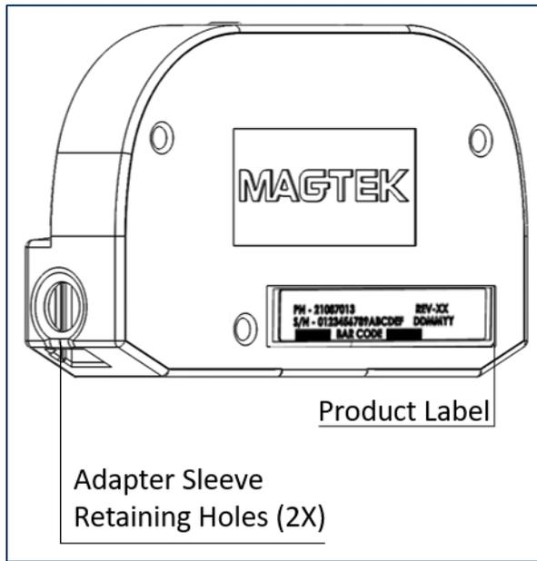
**Figure 1-2 - iDynamo 5 Gen III Major Components (Back)**
